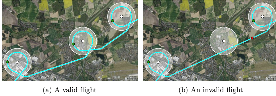
Fig. 2: Traces of drones monitoring closeness to celltowers.
