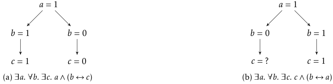
FIGURE 2.5: Two BDT that represent the Skolem functions for the respective QBFs below.
