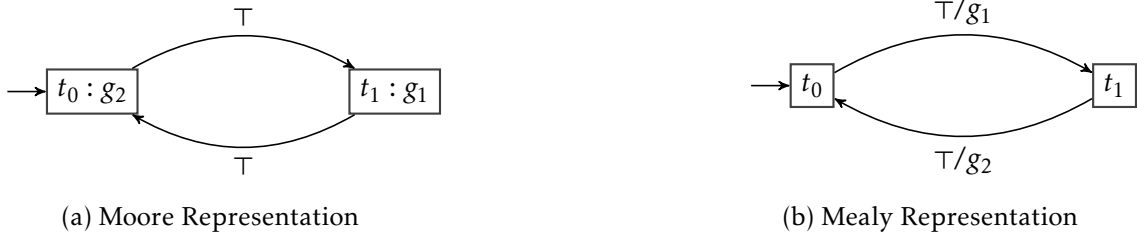
FIGURE 2.2: A virtual representation of the transition systems \langle T, t_0, \tau \rangle with input set \{r_1, r_2\} and output set \{g_1, g_2\} , with: T = \{t_0, t_1\} and \tau = \{(t_0, \top, \{g_1\}, t_1), (t_1, \top, \{g_2\}, t_0)\} , where \top accepts every input.
