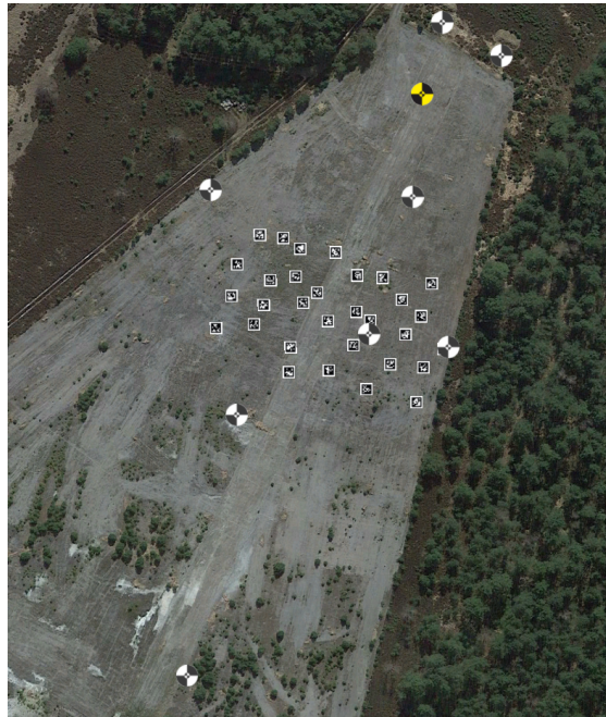
Figure 5.2.: A representation of the landmarks used for visual navigation in the test flight.
