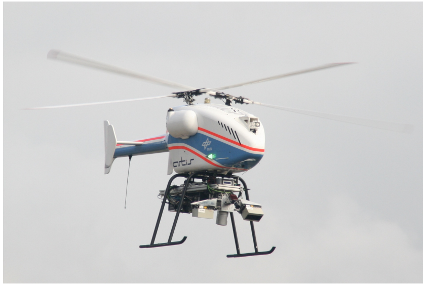
Figure 5.1.: Picture of the helicopter that is used for the flight test. This vehicle has a total mass of 150kg and a payload up to 85kg. The high payload allows besides the sensors needed for the flight execution also additional hardware like the board running the hardware monitor.
