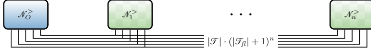
Fig. 4: Overview of the parallel approach : The n subnets are connected such that for every transition t \in \mathcal{T} there are (|\mathcal{Y}(t)| + 1)^n transitions, i.e., there is one transition for every combination of which transit of t (or none) is tracked by which subnet. We use until operators in the constructed LTL formula to only skip steps not involving the tracking of the guessed chain in the flow formula.
