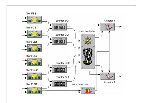
Fig. 3. System diagram of the SLS controller.
