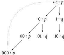
(The dotted line means that the same tree would repeat there. Note that, in general, an alternating automaton may also have more than one run on a particular word—or no run at all.)
