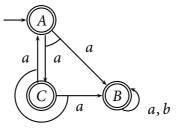
• Alternating automaton, both branching modes (arc between edges indicates universal branching mode),  $L = aa(a + b)^{\omega}$
