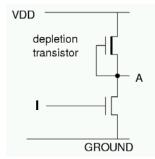
Depletion transistor (resistor) contributes a weak value to be considered in the #-operation for signal A
