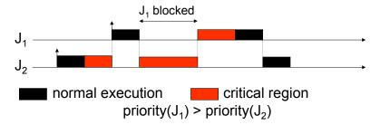
Here: Blocking time equal to length of critical section.
