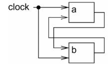
• In an actual clocked (synchronous) hardware system, both registers would be swapped as well.
