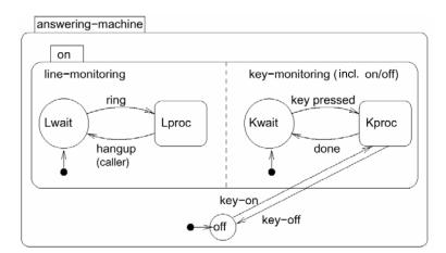
Line-monitoring and key-monitoring are entered and left, when key-on and key-off events occur.
