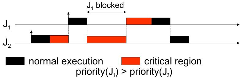
■ Here: maximum blocking time of J₁ equal to length of critical section of J₂.
