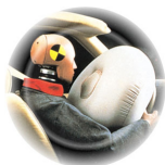
Sideairbag in car, Reaction in <10 mSec
