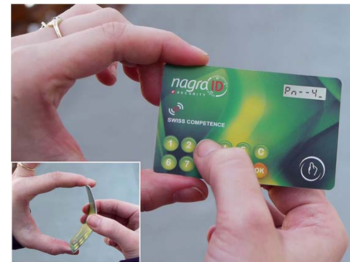
smart card with numeric key pad and display (NagraID, 2010)
