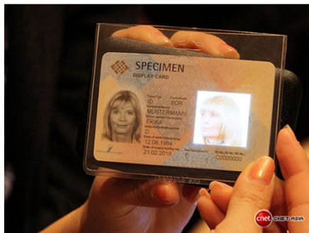
smart card with OLED display (Samsung, 2010)
